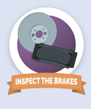
Your brakes should be checked at least twice a year to ensure safety. If there's 4 millimeters or less of friction material remaining, your brakes should be replaced.
