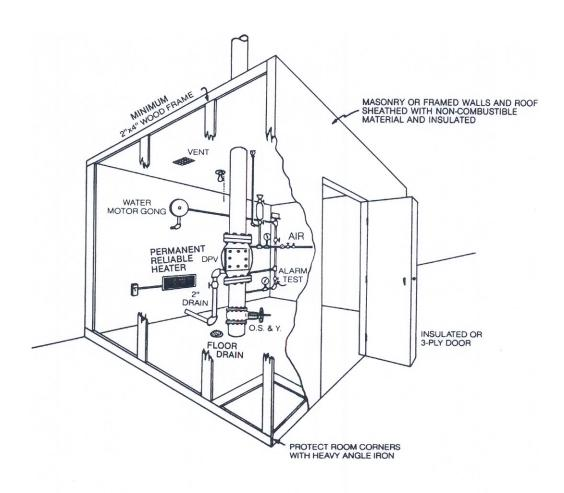
IF CONCEALED OR CRAWL SPACES EXIST BELOW FLOOR LEVEL, ADDITIONAL PROVISIONS ARE NEEDED TO PROTECT THESE AREAS FROM FREEZING TEMPERATURES
